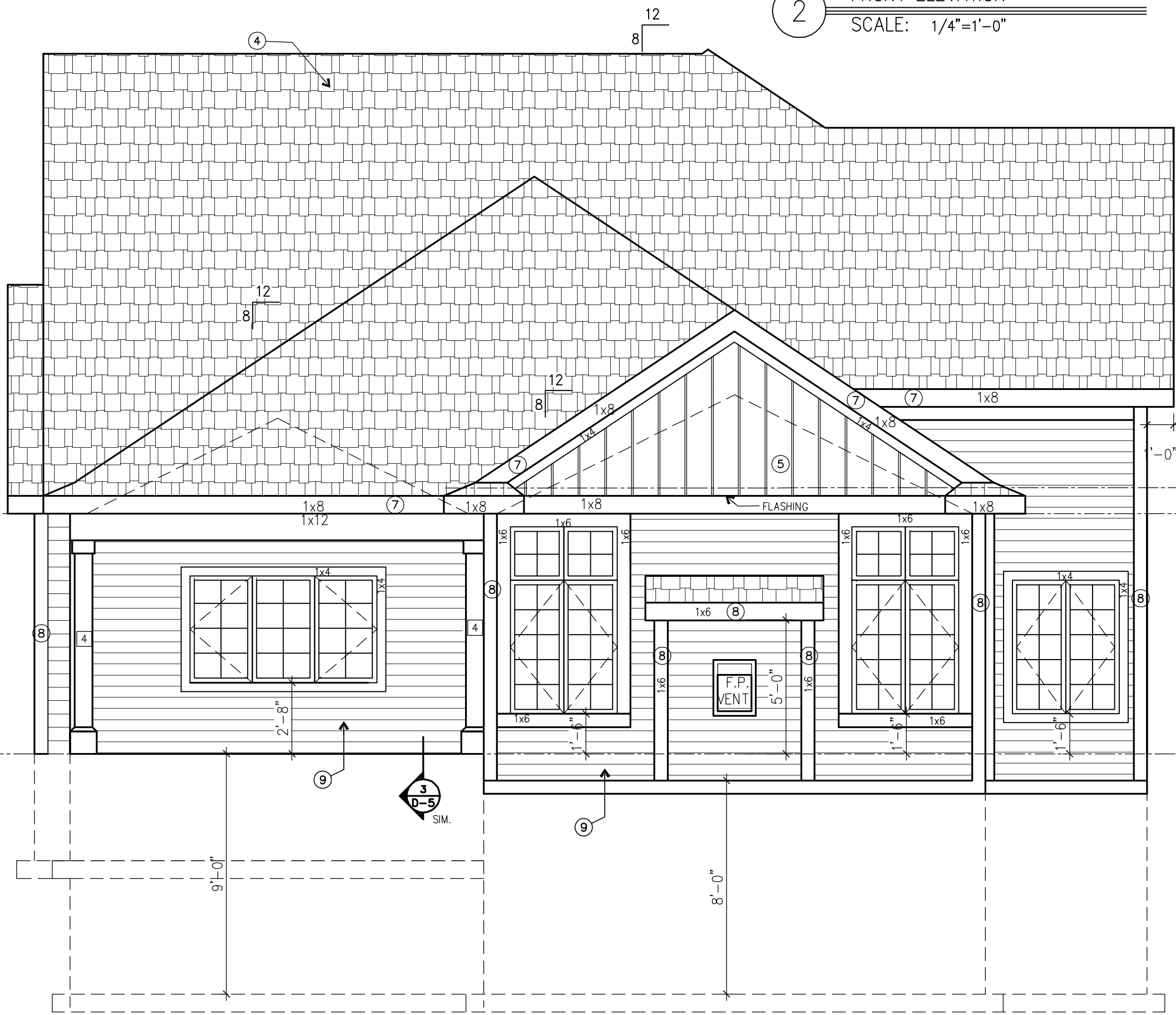
1 REAR ELEVATION SCALE: 1/4"=1'-0"
